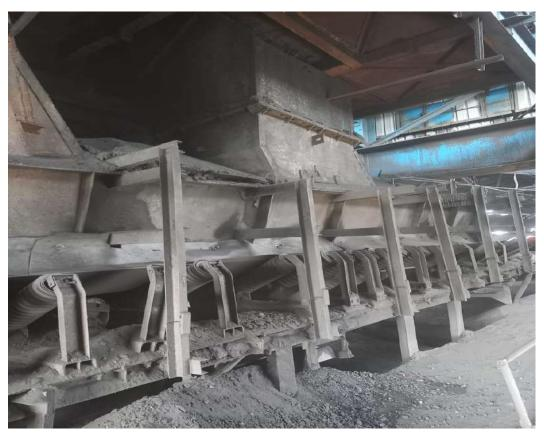
Considering long service life minimum 15 years, shuttle conveyor needs to be renovated and modernized for smooth running of coal handling plant for smooth generation by complete replacement of travel rail track system with modified system, modification of deck module by reducing load on shuttle gross weight, replacement of deck sheets, modified take up tensioning arrangement etc.
